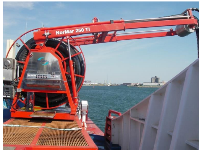
Fig. 22 Hydraulically driven reel with 360° turntable, umbilical hose and integrated crane
