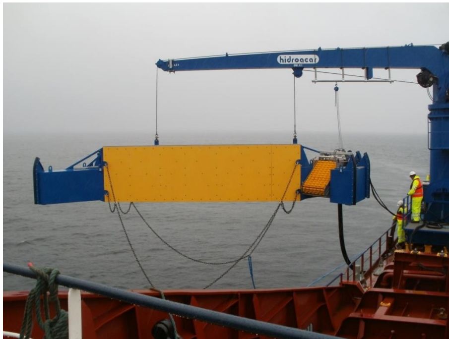
Fig. 1 LAMOR Stiff Sweeping Arm system LSS 12m
