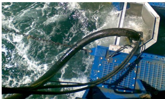
Fig. 6 LSS 12m, oil hose connected to weir skimmer module
