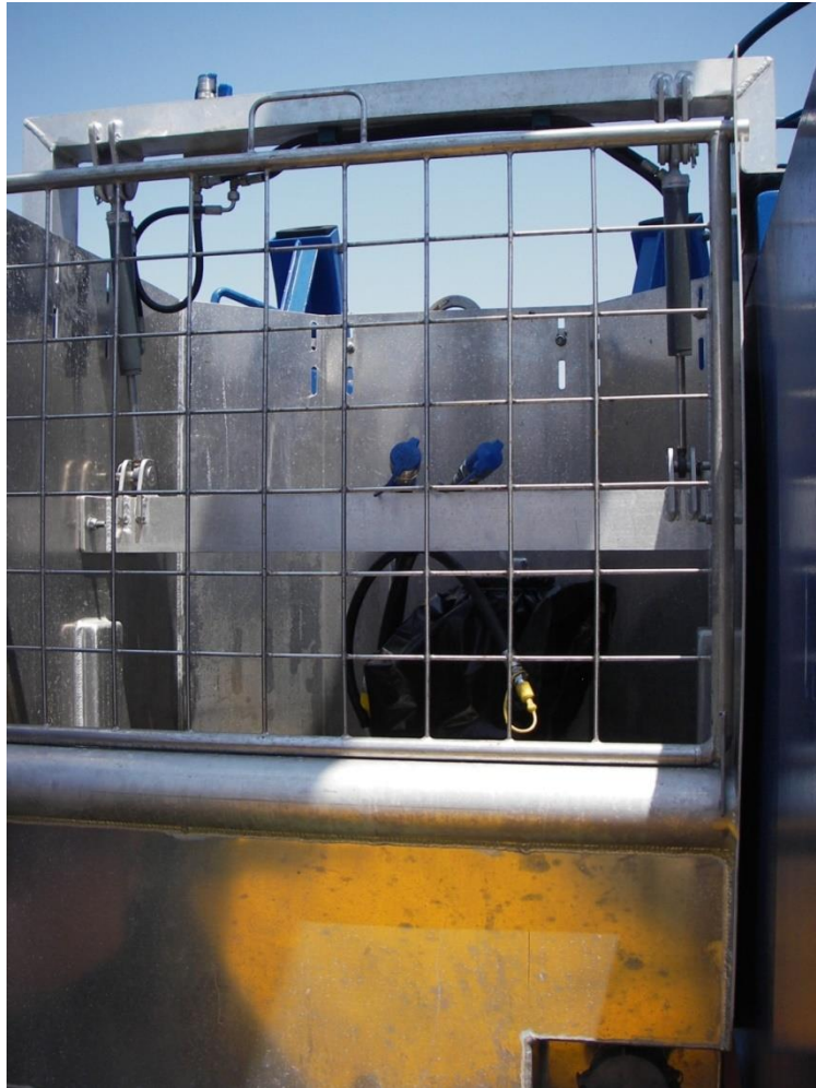
Fig. 2 LAMOR Stiff Sweeping Arm LSS 12m – weir skimmer module with debris screen
