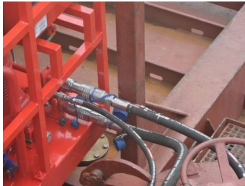
Fig. 25 Hydraulic hoses set connected to NorMar DHHP
