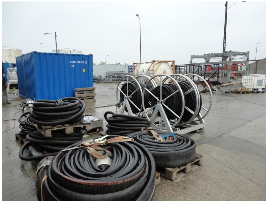
Fig. 7 Hose Winders LHW 40/2-AL with hydraulic hoses for LSS 12m
