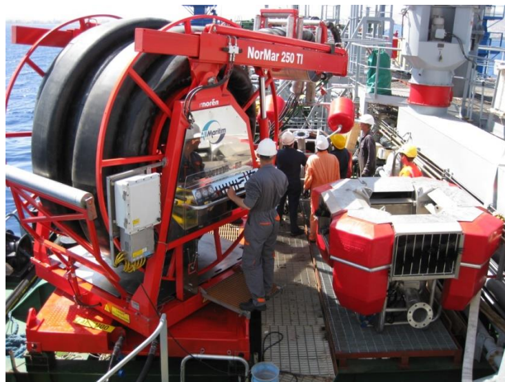
Fig. 17 NorMar 250 TI High Capacity Skimmer Set. Brush/disc skimmer head.
